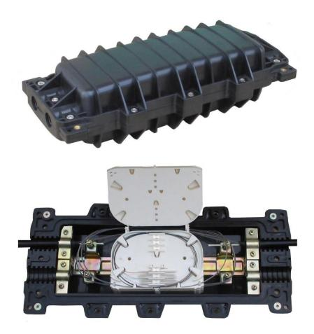
FOSC-001 provide with 4 fiber cable in-out round ports and the cable diameter is from  $\Phi 10-\Phi 22$ . It can be used in aerial, duct, and direct buried application. This product is made from the high-quality and with the mechanical sealing structure filled with the sealing material. The external component and fastening piece are all made from the high-quality stainless steel. It can be opened after sealing.
